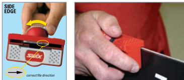
Generally 1 to 3 degrees resulting in a total edge angle of 87 to 89 degrees.
