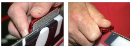
Removing burred steel from filing with a diamond stone
