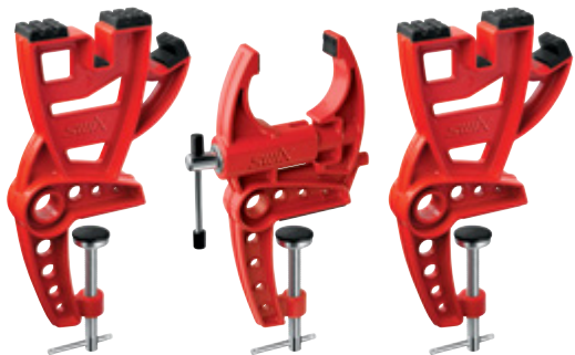
T0149-20 JAW ECONOMY VISE Three pcs. vise with jaw fixation. 20 mm wide jaws. Opens from 35 mm to 90 mm. 60 and 90 degrees side edge working position. Light weight and compact. Ea.
