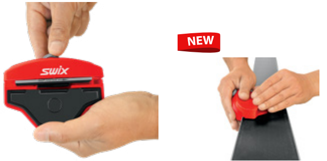
TA3006 MULTI EDGER The Swix multi edger tool is all you need to sharpen and bevel your edges. You can set up the base and side edge in one tool! Dial a precise side angle from 0 to 5 degrees and 0.5 to 1.0 degrees on the base—nine different angles in total. Always set the base edge angle before the side edge angle. We add a bevel to the base edge to make the skis more predictable or forgiving and bevel the side edge to give more grip on hard snow and ice.
